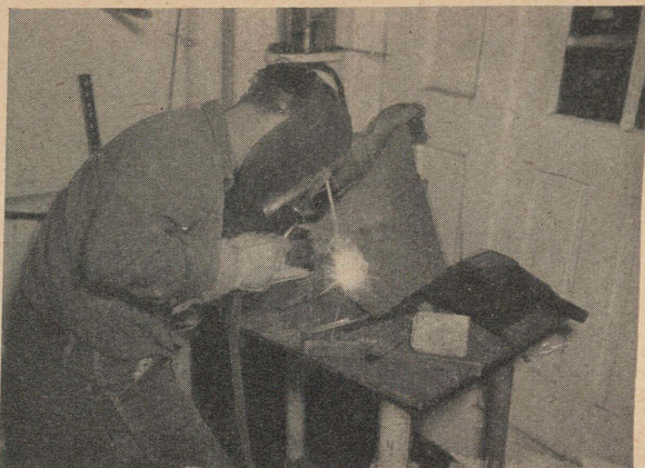
PLATE 5—FIGURE 1.—Training in above-water burning as a prelude to under-water cutting.
