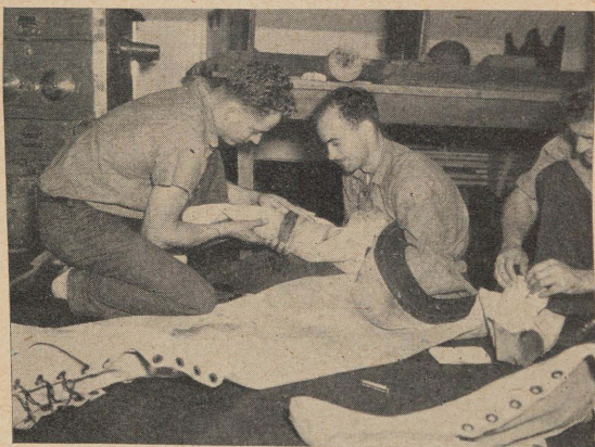
PLATE 5—FIGURE 2.—Diving suit repair work.
