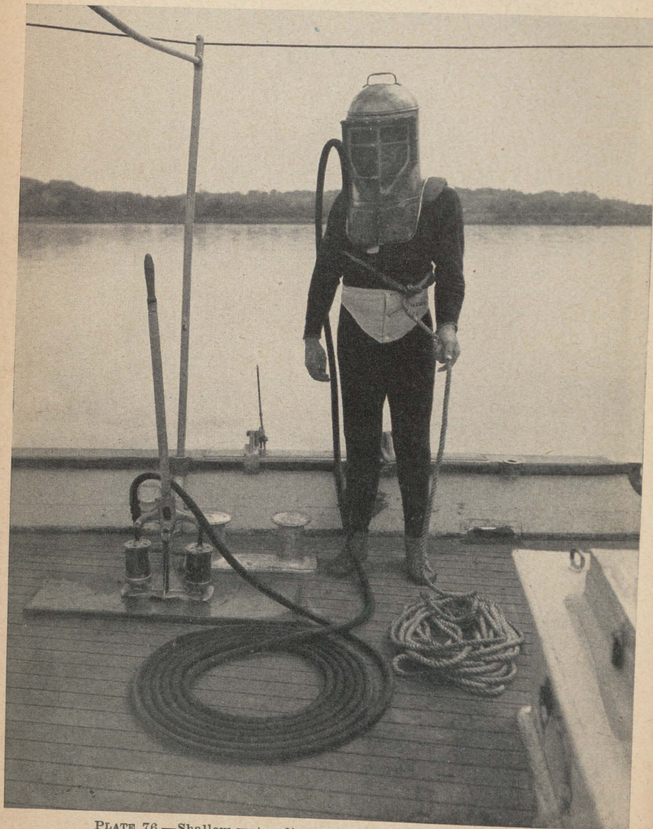
PLATE 76.—Shallow water diving apparatus—Miller-Dunn type.
