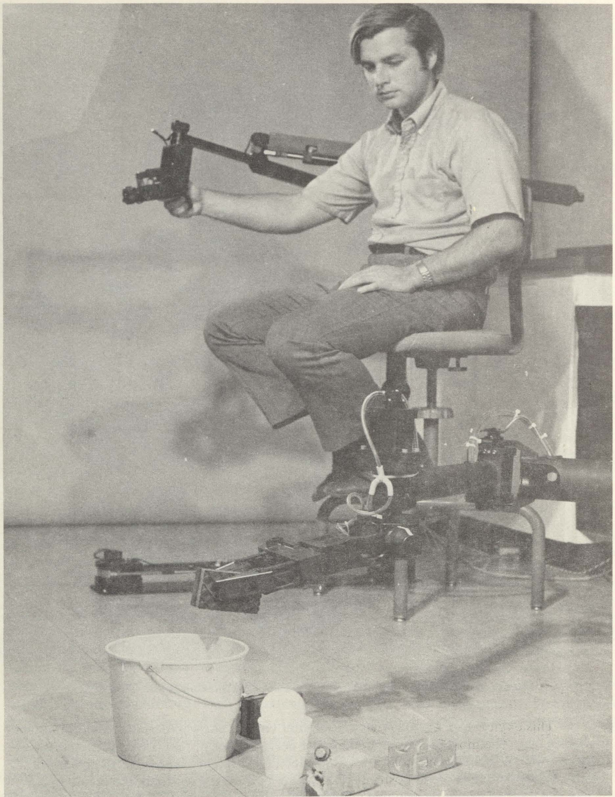
Figure 14. Controller and main RUWS manipulator during laboratory testing. 2588-3-72
