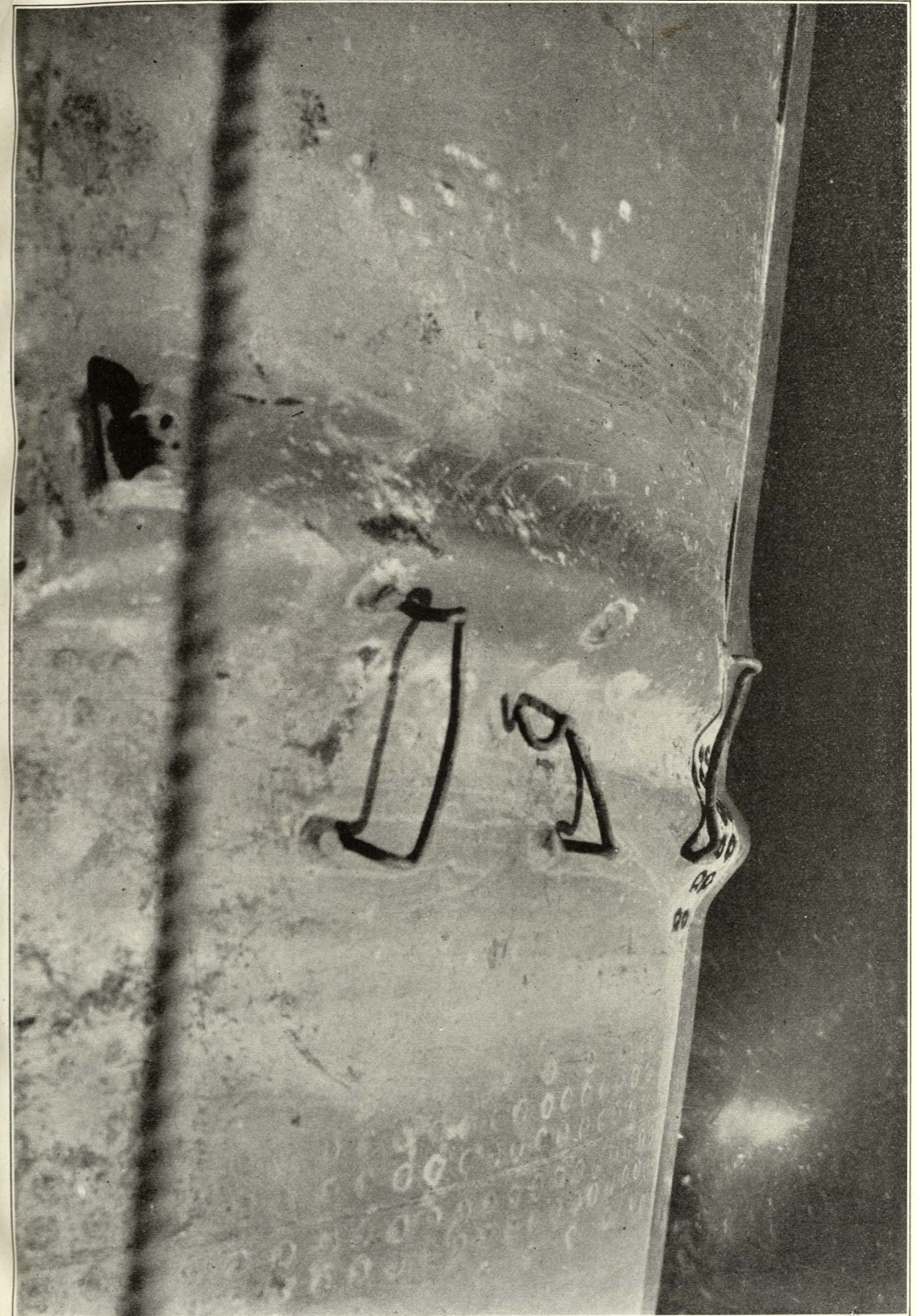
FIG. 40.—PORT SIDE VIEW SHOWING WRINKLE CAUSED BY BOW STRIKING BOTTOM AFTER COLLISION WITH "CITY OF ROME"
