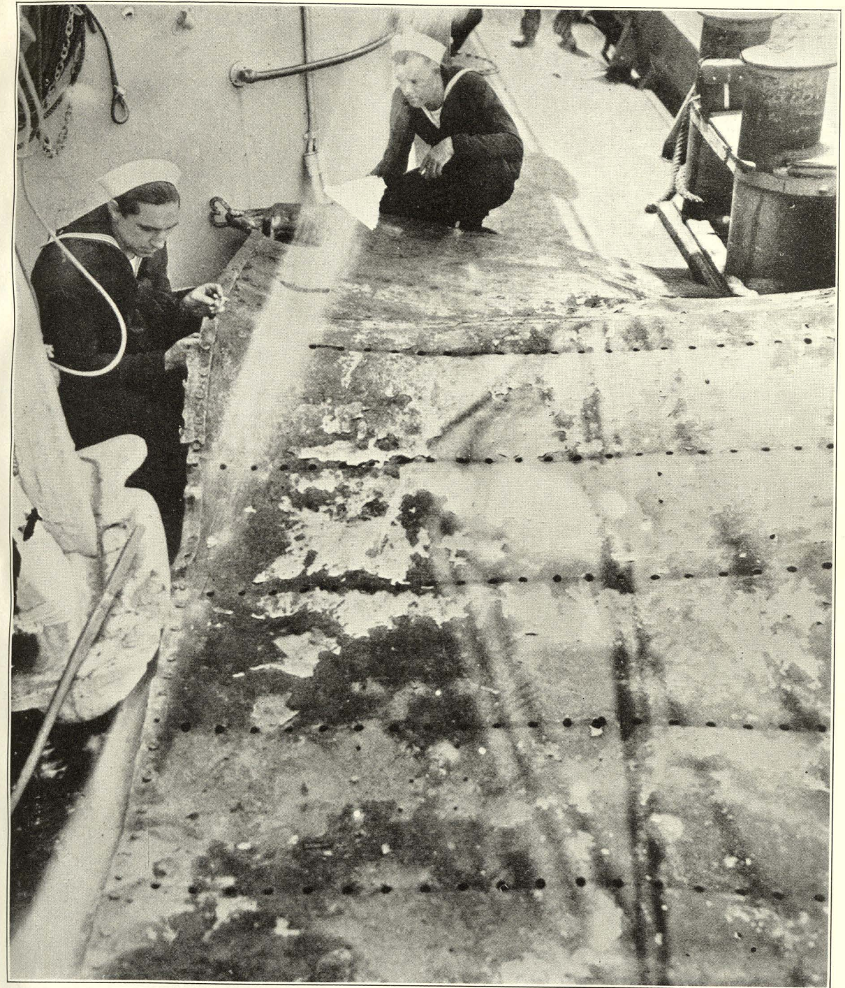
FIG. 42.—"S-51" BOW PLATING AND STEM CASTING ON BOARD "SAGAMORE"
