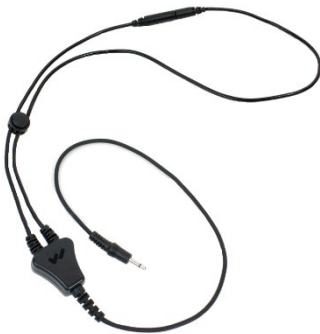
Figure 2. Neck loop. Works with Tcoil-equipped hearing aids and implants.
