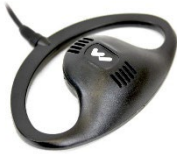
Figure 5. Over-ear speaker. Not compatible with TCoil. Hearing aid not required.
