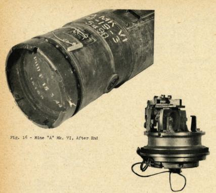
Fig. 17 - Detonator Hydrostat, Mines "A" Mks. VI-VII
