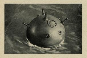
Fig. 28 - Mine Type GR, Floating
