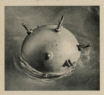
Fig. 50 - Mine Type GZ, Floating
