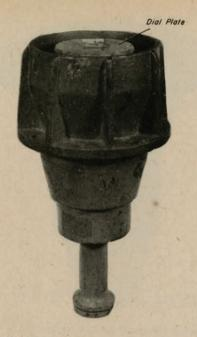
Fig. 10 - Depth Charge Pistol Type V
