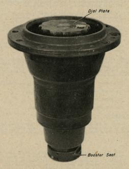
Fig. 5 - Depth Charge Pistol Type II, Top View
