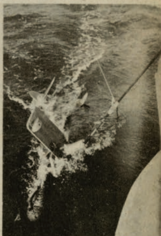
4. RELEASE PELICAN HOOK WHEN DETECTOR CLEARS SHIP
