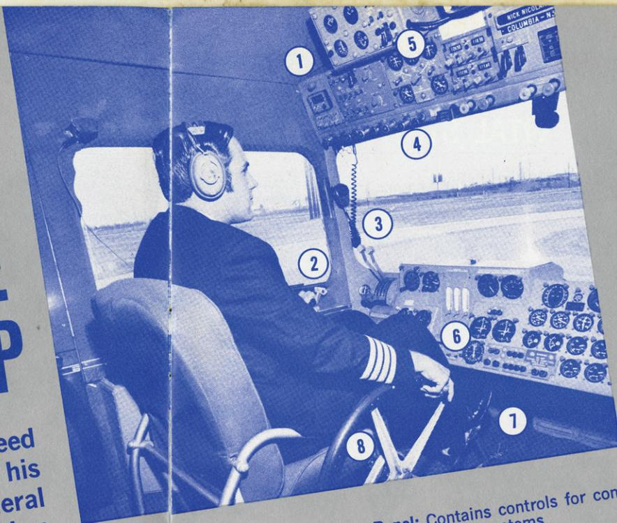
1. **Overhead Control Panel:** Contains controls for communications, fuel and electrical systems.
