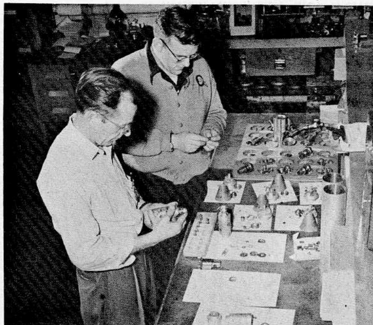
BREAKDOWN AND INSPECTION OF FUZE COMPONENTS
